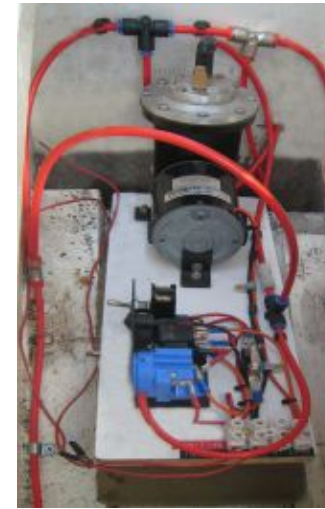
The prototype vacuum pump installed in one of the coaches for testing.
