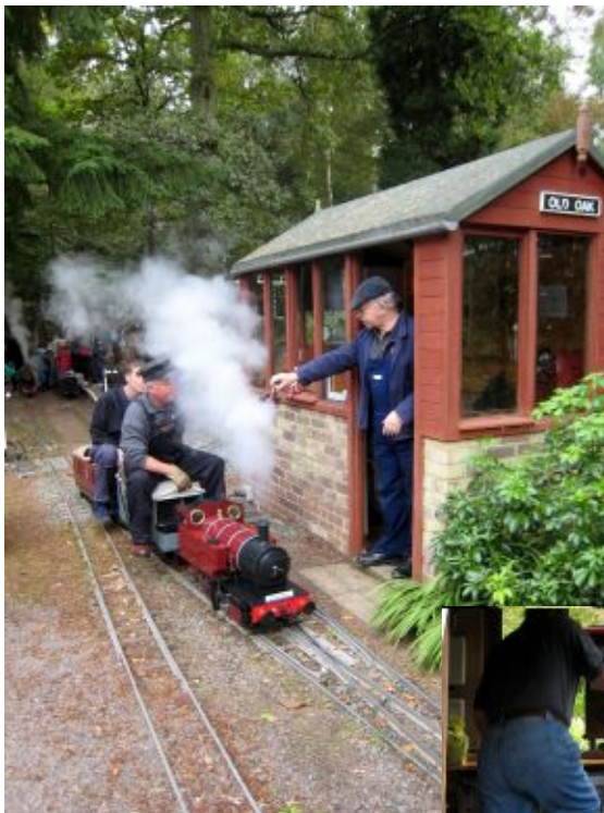
Receiving the token for single line working at Old Oak signal box.
