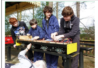
Photo Paul Konig. Assembling the wiring into the Titan 7 chassis.
