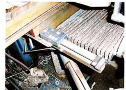
5 Left: A linear scale on the z axis (Also visible is the original MPS unit on the x axis) 6 Above: A linear scale on the y axis
