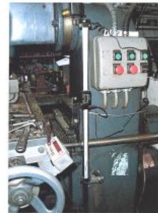
5 Left: A linear scale on the z axis (Also visible is the original MPS unit on the x axis) 6 Above: A linear scale on the y axis
