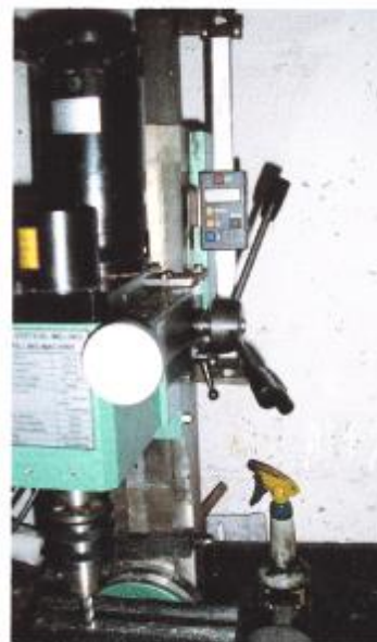
Linear scales fitted to the x and z axes of a small Warco mill. (The y axis is also fitted.)
