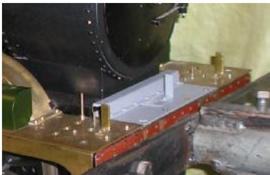
Showing the start of the work for the front sanding boxes. The cross shaft will pass through the prototypical square section tube added in front of the smoke box.
