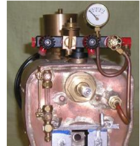
The new steam fountain and back-head fittings, including the water gauge.
